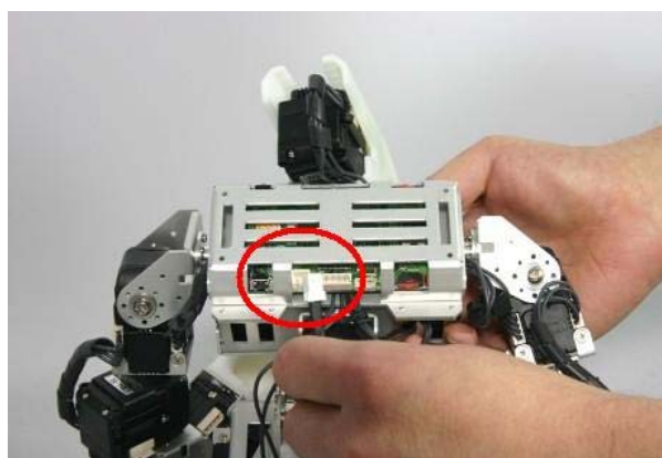
< Exterior power connection >
